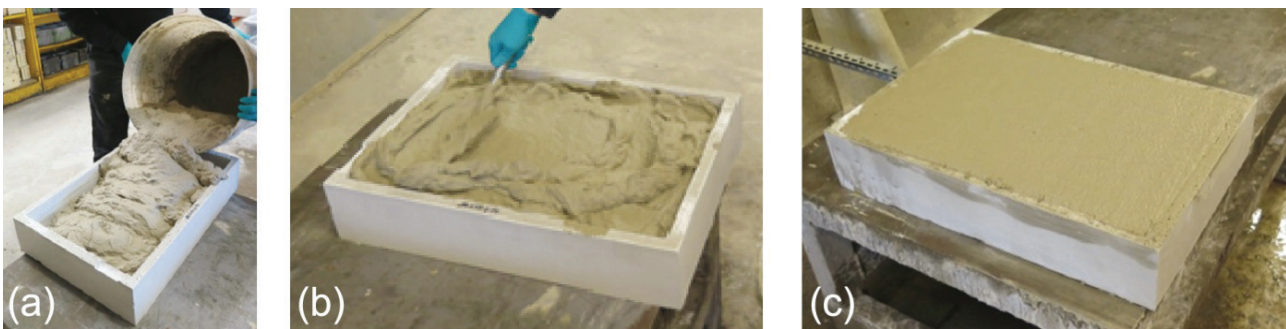
Fig. 11. Manufacturing of small-scale UHPC-CLC elements. (a) Cast of CLC; (b) Distribution of CLC in the UHPC box; (c) CLC after finishing.
