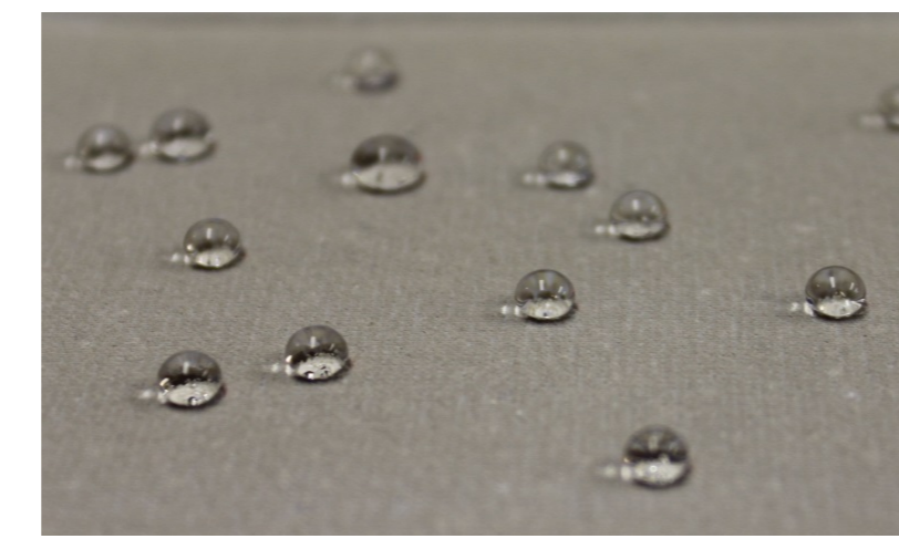
▲ Super hydrophobic surface of UHPC elements, © BAM
