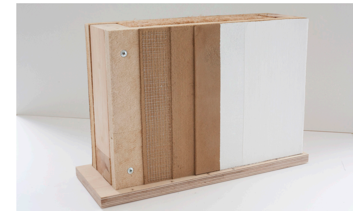
◀ 1:1 Sample wall build-up showing single layers and connection means
